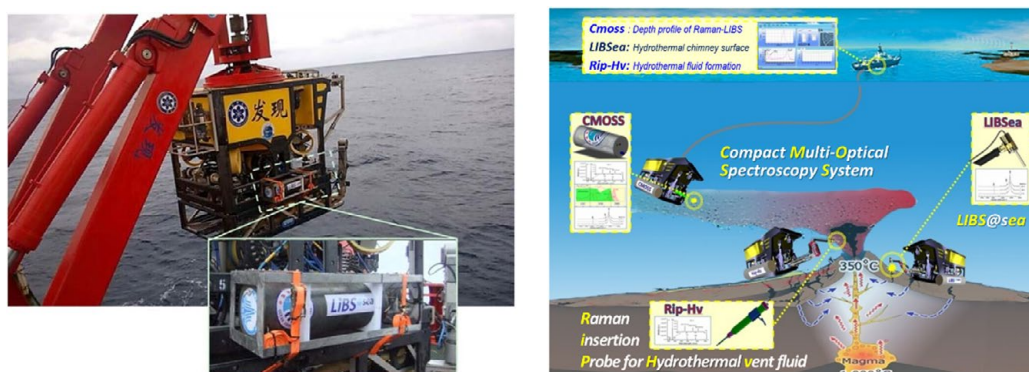
Fig. 1: A deep-sea LIBS system deployed on the ROV of “Faxian” (left) for the sea trial in 2015, and a concept diagram (right) showing the hybrid spectral system and its possible applications to hydrothermal vent.
